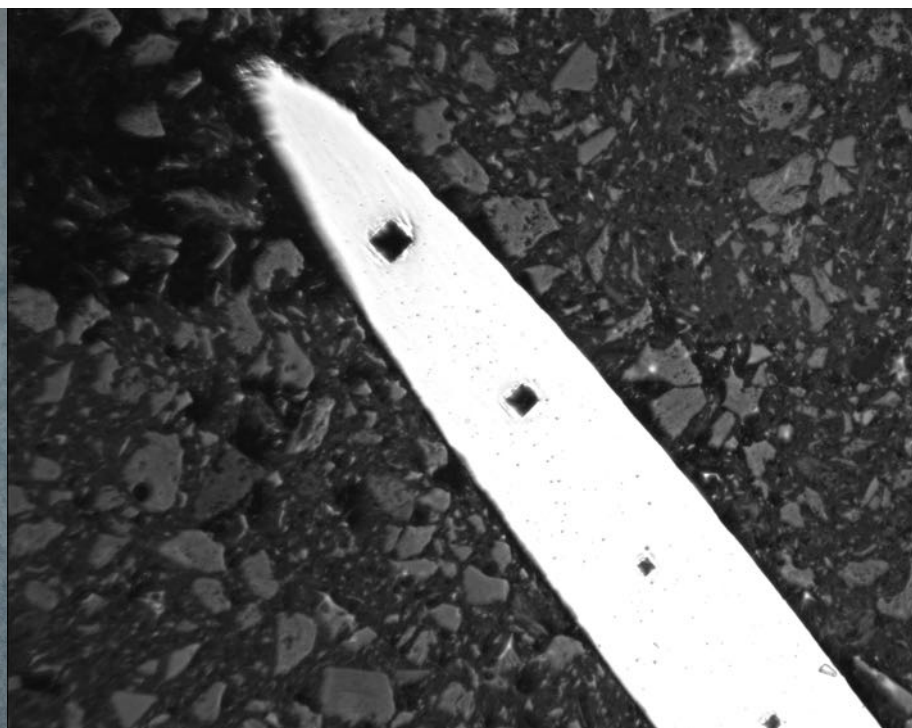
Figure 14: Sample Undergoing Hardness Test
